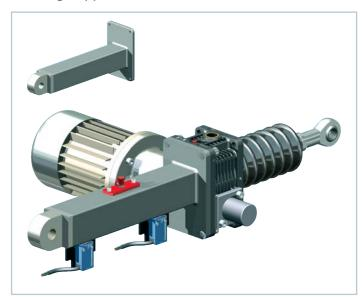
The **pivoting support tube STRO** has the advantage that the pivot points are entirely external. The disadvantage is that the gearbox and motor weights are in the centre. The manufacture is always customer-specific.
