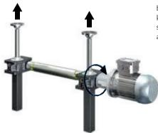
Check the direction of rotation required for the system and record this on the drawing or select one of our standard system layouts (Checklists). With T bevel gearboxes, the direction of rotation can be changed simply by turning the gearbox around.
