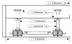
Screws and guides must be parallel to each other, otherwise the equipment can seize up during operation. All mounting surfaces for the gearboxes must be exactly at right angles to the guides, jamming may occur, leading to rapid wear and/ or serious damage. Squeaking noises can also occur on R versions. We recommend aligning with the help of a precision machine spirit level. The mounting surfaces for the nuts must also be at right angles.
