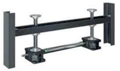
Attention must be paid to the parallelism and correct angular relationships of mounting surfaces, gears, nuts and guides to each other. The same applies for exact alignment of gears, pedestal bearings, connecting shafts and motors to each other. We recommend aligning with the help of a precision machine spirit level.
