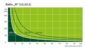
These curves are for guidance under standard industrial conditions (ambient temperature 20°C etc.) and correct maintenance (lubrication etc.). They are based on the ZIMM standard trapezoidal thread Tr 140x20. The operation cycles can be many times longer, when using ball screws.
